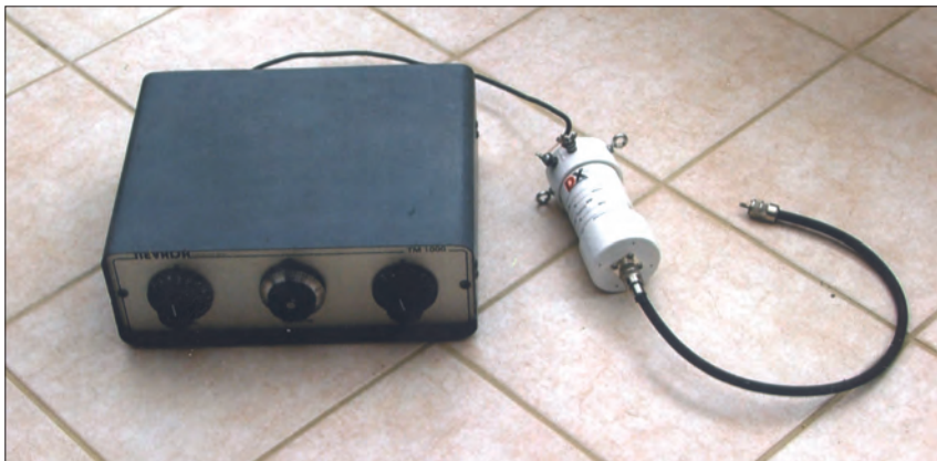
Fig. 3: The commercial and physically small choke balun should be fitted close to the single-ended a.t.u. to be effective. A simple multi-turn coil made up of extra coaxial cable could be just as effective. See text for more detail.
